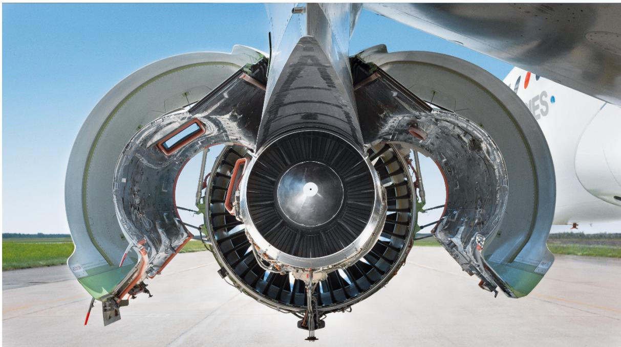
Open turbine with turbine disk. Source: MTU Aero Engines.
