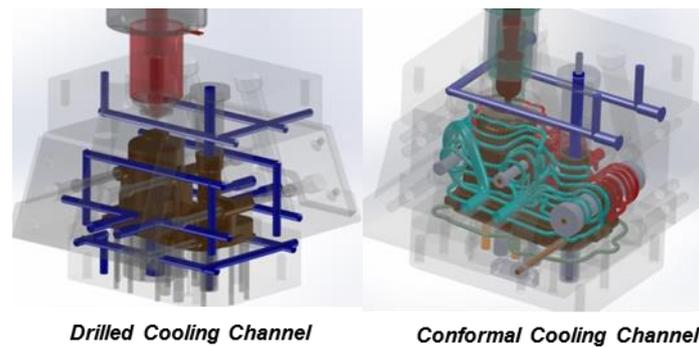
Figure 5 – Comparison in cooling channel design: former mold with drilled cooling channels and new mold with conformal cooling channels
